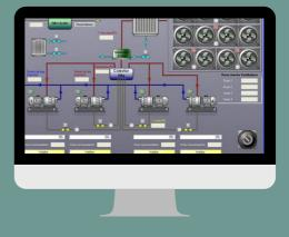
Power management is fully integrated into the software. Engines are continuously going to the ideal position for maximum energy efficiency in combination with self declared priorities. This increases the service life of compressors considerably. Several peak shave options to reduce the maximum electricity consumption/hour are available in the program.
